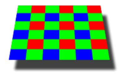
Photo receptors on the digital camera sensor are arranged in a matrix and covered with color filters so each can record red, green or blue colors (bayer pattern).
