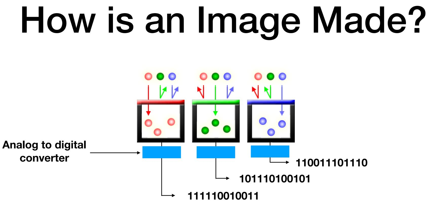
The amount of light that reaches each receptor generates a corresponding electrical charge which is converted to a digital representation through an analog to digital converter.
