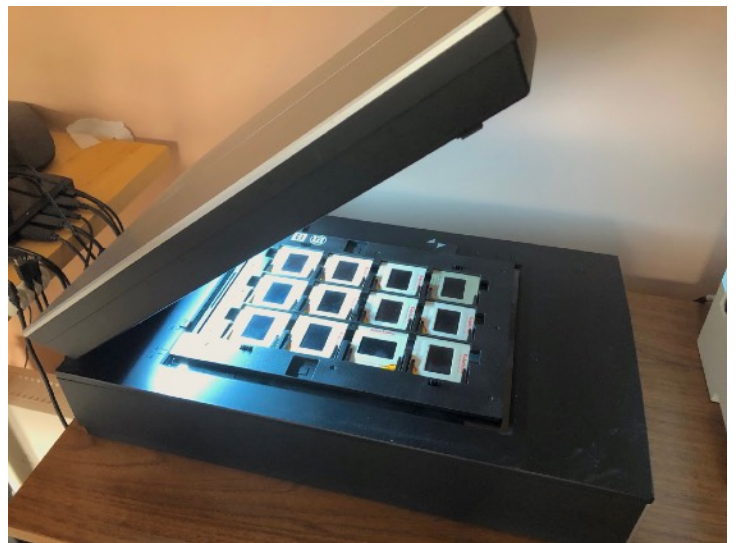
Transparency unit includes a separate light source above film with sensor below.
